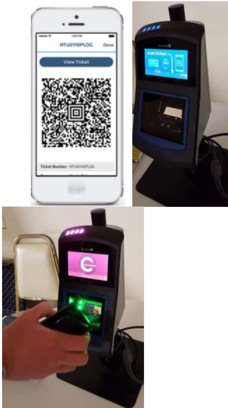
Figure 1: QR Ticket Sample from Masabi and Onboard Ticket Validators and NFC Technology from ACCESS-IS
