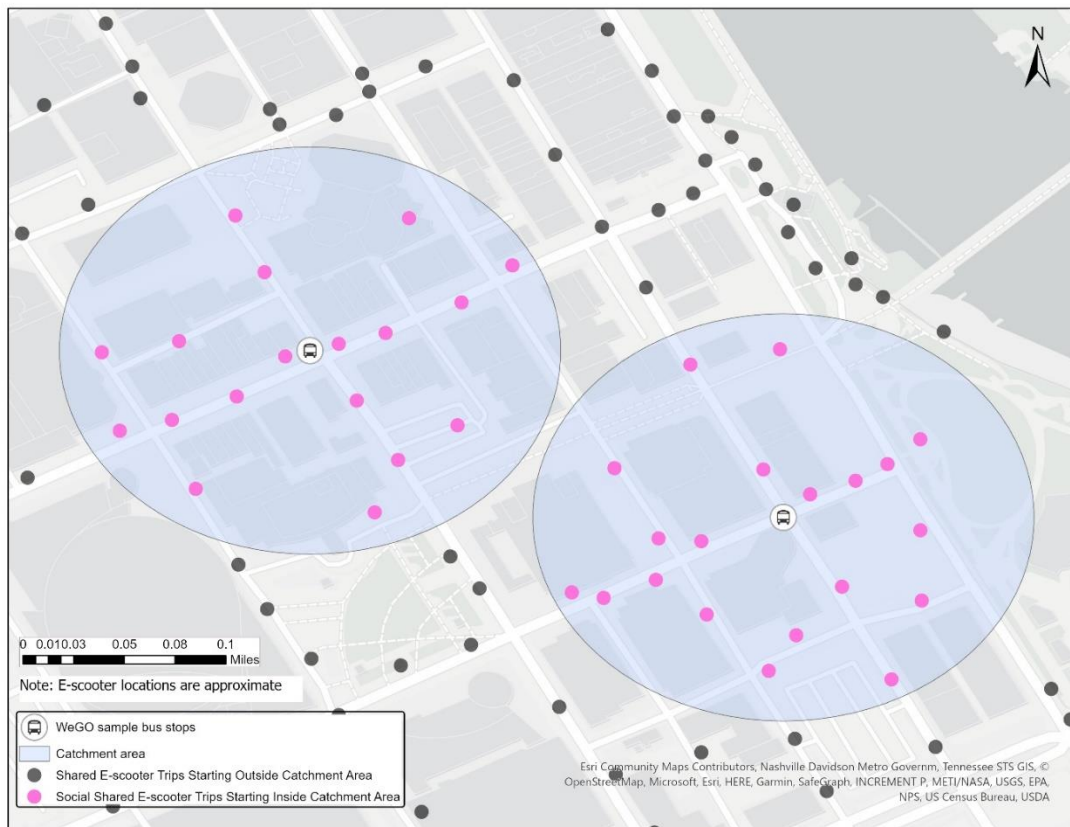
12 13 Figure 3: Example of shared e-scooter trips assignment method to bus stops
